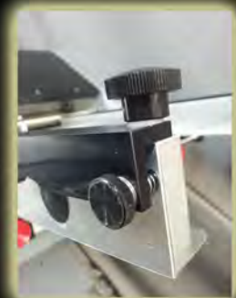
Easy Skew adjustments for squaring the stock.
