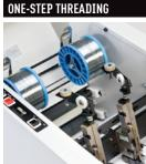
Magnetic stitching heads feature one-step threading for quick and easy set-up.
